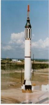
The Mercury-Redstone Launch Vehicle, designed for NASA's Project Mercury, was the first American manned space booster. It was used for six sub-orbital Mercury flights from 1960–61; culminating with the launch of the first, and 11 weeks later, the second American (and the second and third humans) in space.
